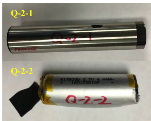
FIGURE 21. Lithium-ion battery inside e-cigarette.
