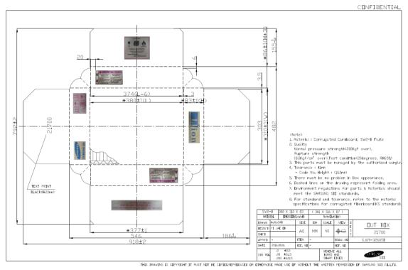
Fig. 2-1. Outer box package drawing.
