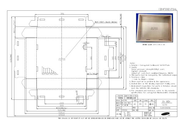
Fig. 2-2. Inner box package drawing.
